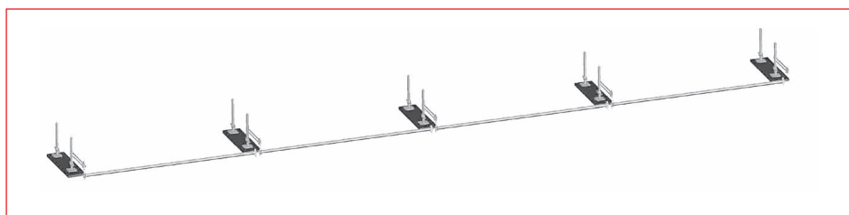
Fig. 3.52 – Step 1 – Footing assembly
