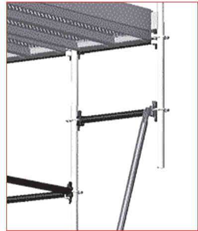
Rys. 3.29 – Platform expanded with the transoms and braces
