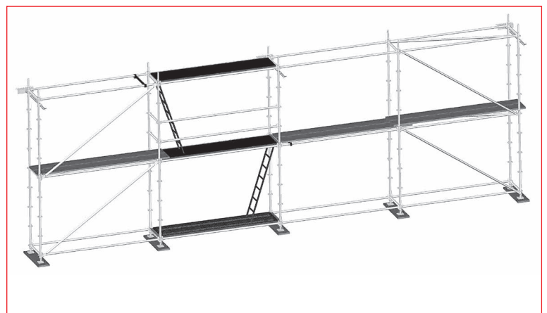
Fig. 3.59 – Example showing the scaffolding anchored to the facade
