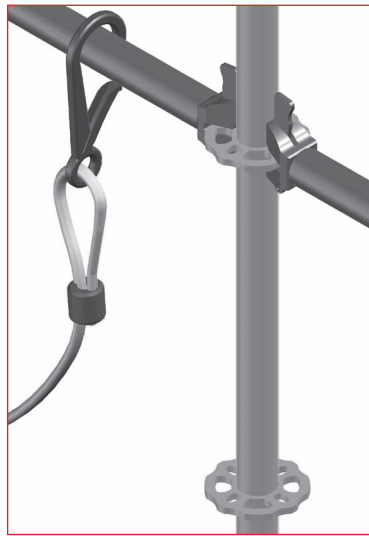
Fig. 3.9 – Attachment to the transom
