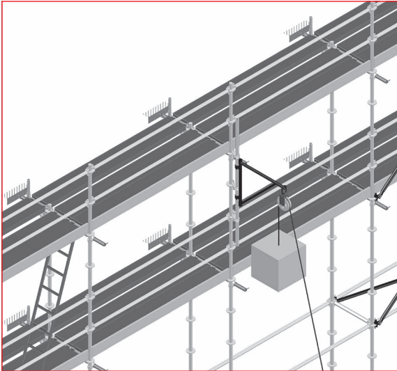
Fig. 3.79 – Scaffolding with the winch
