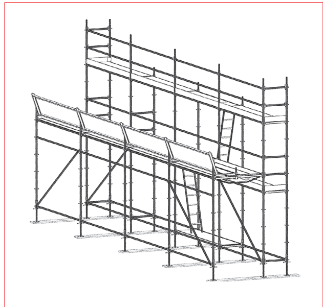
Fig. 3.38 – Example of a circulation path for pedestrians
