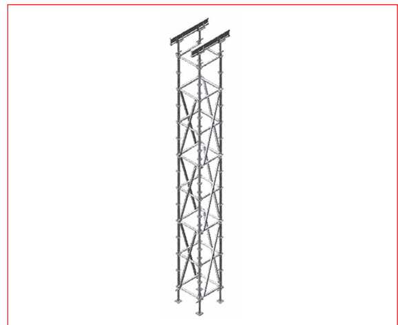
Fig. 3.64 – ROTAX Plus scaffolding in a tower set-up
