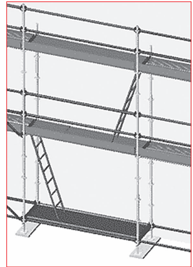
Fig. 3.41 – Scaffolding entrance with passing aluminium platforms fitted with the aluminium ladders
